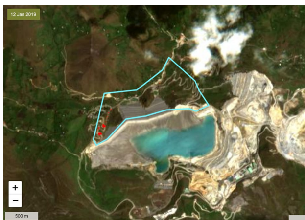
Fig. 10 Example of change in NDVI for a tailings dam in Peru on 12 Jan 2019, based on a comparison between the first clear day post-incident image and three pre-incident images. The spill occurred on 16 Dec 2018 from the left side of the dam
